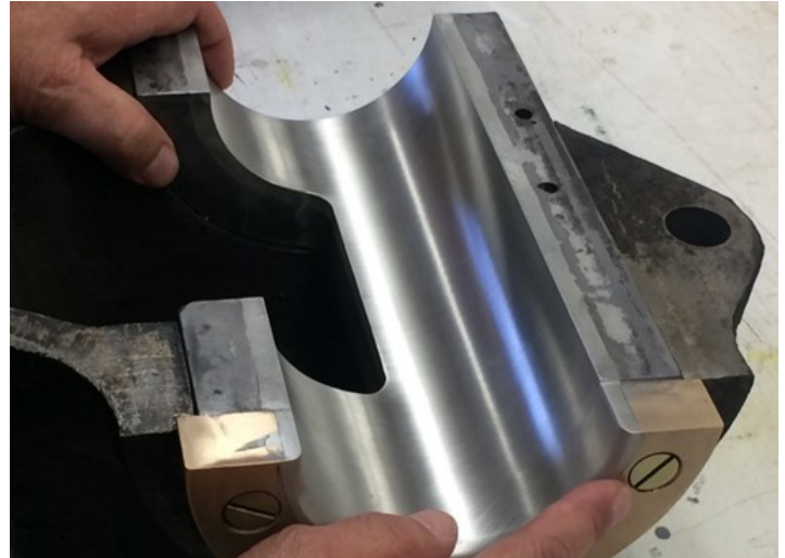
Re-babbitted axle bearing for Connecticut Car 838
